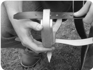
Slot the ankle strap through the angle frame.
