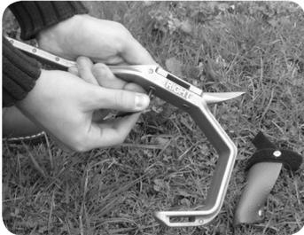
Remove the leather protective cover and screw the spike into the angle frame.
