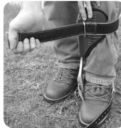
Tighten the shin strap to fit your leg using the self gripping srtp.
