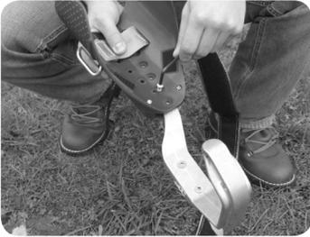
Screw the shell onto the angle frame (to ensure optimum hold, position the screws as far apart as possible).
