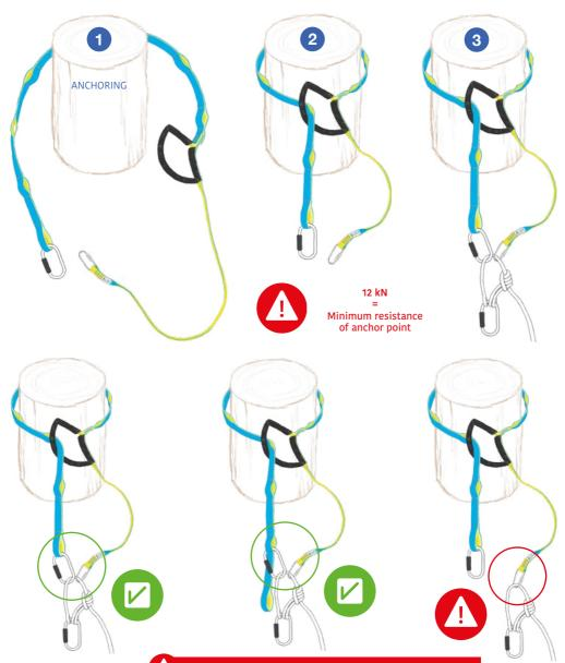
THE USER'S CLIMBING ROPE MUST ALWAYS BE CONNECTED TO THE MAIN ANCHOR OR TO AN INTERMEDIATE ANCHOR.
