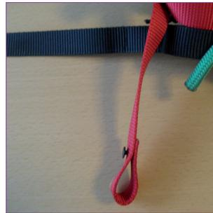
11. Insert the lower rivet part through the folded up strap and connect it to the upper rivet part it to the upper rivet part.
