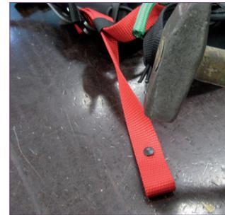
12. Place the strap on a solid surface, and use a hammer to drive the rivet into place. Repeat the assembly steps shown in pics 1 to 12 for the second Hip/Leg connection.
