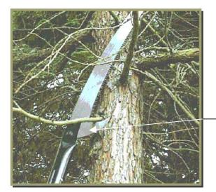
2. Do not cut twigs with sickle blade A. Like sickle blade B, the Hayauchi is not designed to cut by pushing up. Improper use may cause breakdown.
