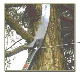
1. Push up the *sickle blade A*, and make a slit in the bark under the twigs
