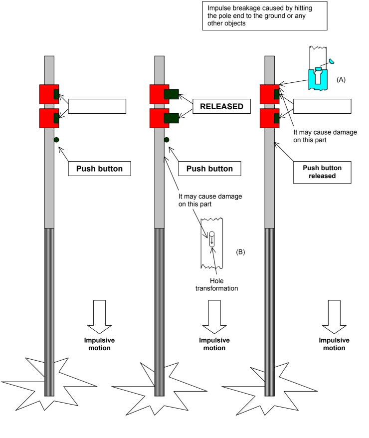
Plastic stopper and push button are set properly. Less breakage but not designed for impulse resistance. Plastic stopper is released which may cause a tear on a part below the push button hole. (B) Push button is released which may cause a breakage on the top part of the pole inside the plastic stopper. (A)
